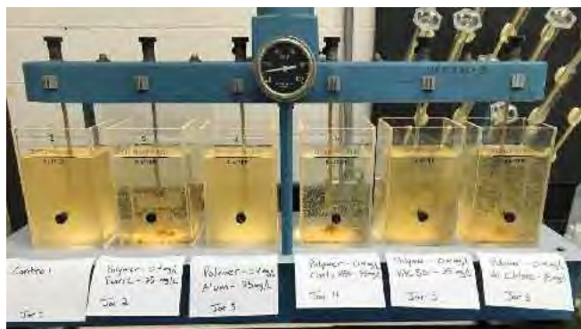
AECOM's assistance in testing different coagulants improved backwash treatment and provided alternatives for treating the backwash wastewater in Sedimentation Basin #5
