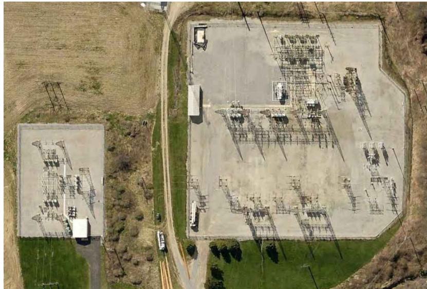
Avangrid initiated a project to upgrade an existing 115/34.5 kV transformer to a higher MVA rating, as well as adding a redundant 115/34.5 kV transformer and associated switchgear, bussing, and controls.
